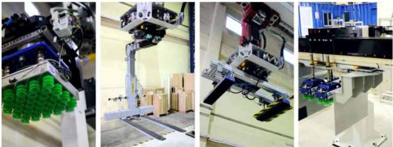
suite of advanced grippers with integrated sensors
