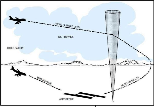
IF IFR, DIVERT OFF AIRWAYS, ESTABLISH VMC AND LAND AT SUITABLE AERODROME OR, PROCEED IN STRICT ACCORDANCE WITH CLEARANCE OR FLIGHT PLAN TO DESTINATION. IF VFR, MAINTAIN VMC TO DESTINATION OR OTHER SUITABLE AERODROME
