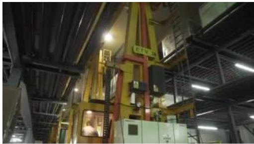
Elevating transfer vehicles will transport, store, and retrieve temperature-controlled containers from SATS' multi-level material handling system.
