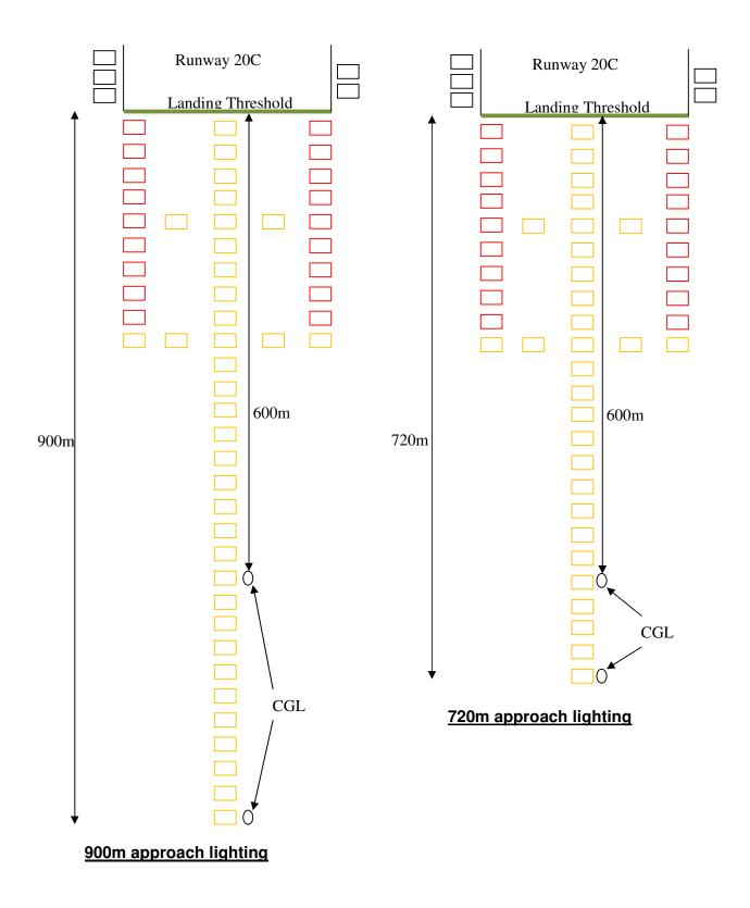
Diagram 1: Illustration of approach lighting (900m versus 720m)
