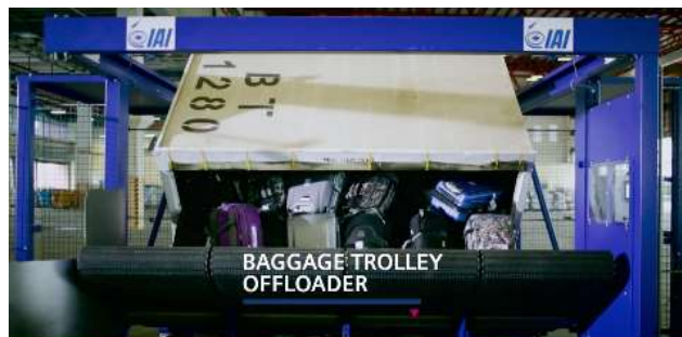
Baggage Trolley Offloader
