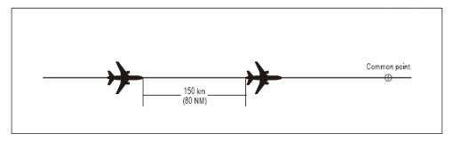
Figure 5-25. 150 km (80 NM) RNAV-based separation between aircraft at the same level (see 5.4.2.5.5 b))
