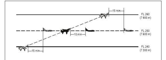
Figure 5-18A. Fifteen-minute separation between aircraft climbing and on crossing tracks (see 5.4.2.2.2.2 a))
