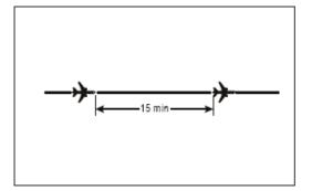
Figure 5-9. Fifteen-minute separation between aircraft on same track and same level (see 5.4.2.2.1.1 a))
