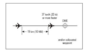
Figure 5-22. 19 km (10 NM) DME or GNSS-based separation between aircraft on same track and same level (see 5.4.2.3.3.1 b))
