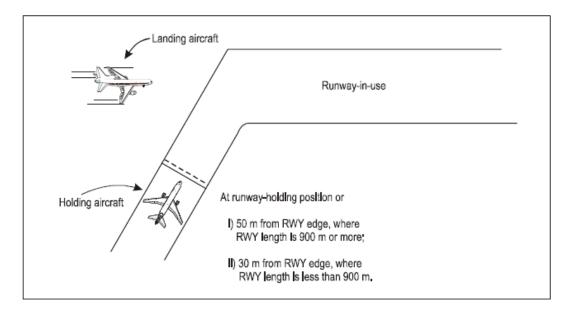
Figure 7-2. Method of holding aircraft (see 7.5.3.1.3.2)
