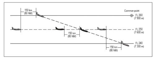
Figure 5-26B. 150 km (80 NM) RNAV-based separation between aircraft descending and on same track (see 5.4.2.5.5 c))
