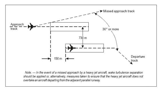
Figure 6-2. Segregated parallel operations where runways are staggered (see 6.7.3.5.2)
