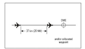
Figure 5-21. 37 km (20 NM) DME or GNSS-based separation between aircraft on same track and same level (see 5.4.2.3.3.1 a))
