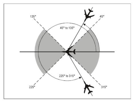
Figure 5-8. Aircraft on crossing tracks (see 5.4.2.1.5 c))
