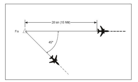
Figure 5-4. Separation using dead reckoning (see 5.4.1.2.1.2 c))
