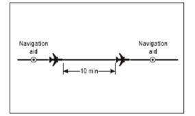
Figure 5-10. Ten-minute separation between aircraft on same track and same level (see 5.4.2.2.1.1 b))
