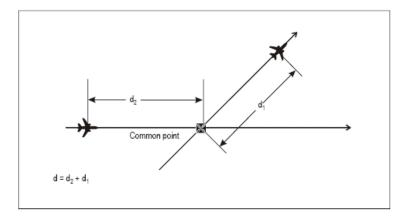
Figure 5-32. Calculation of longitudinal distance between aircraft — opposite sides of the common point (see 5.4.2.6.4.1 b))
