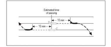
Figure 5-20. Ten-minute separation between aircraft on reciprocal tracks (see 5.4.2.2.3)
