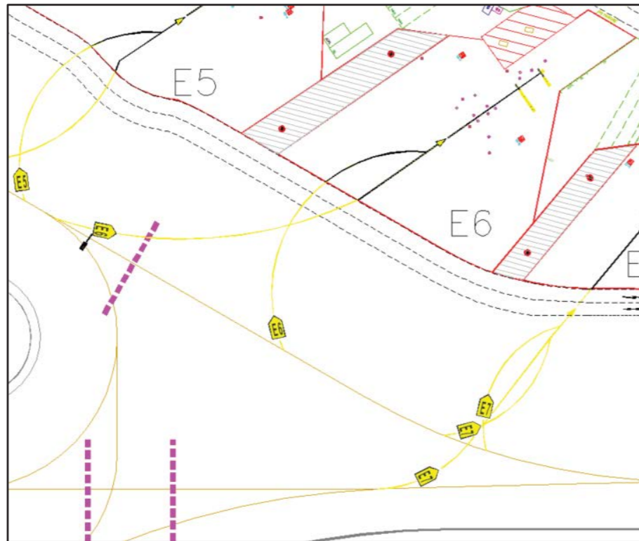
EXISTING AIRCRAFT STAND E6 LEAD-IN LINE AND TAXIWAY/TAXILANE MARKINGS
