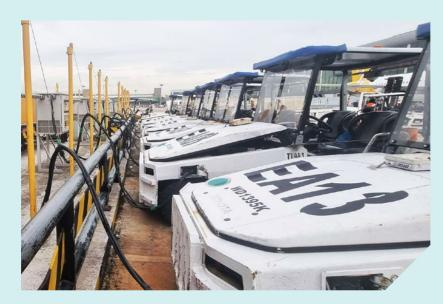
An electric airside vehicle connected to its charging station
